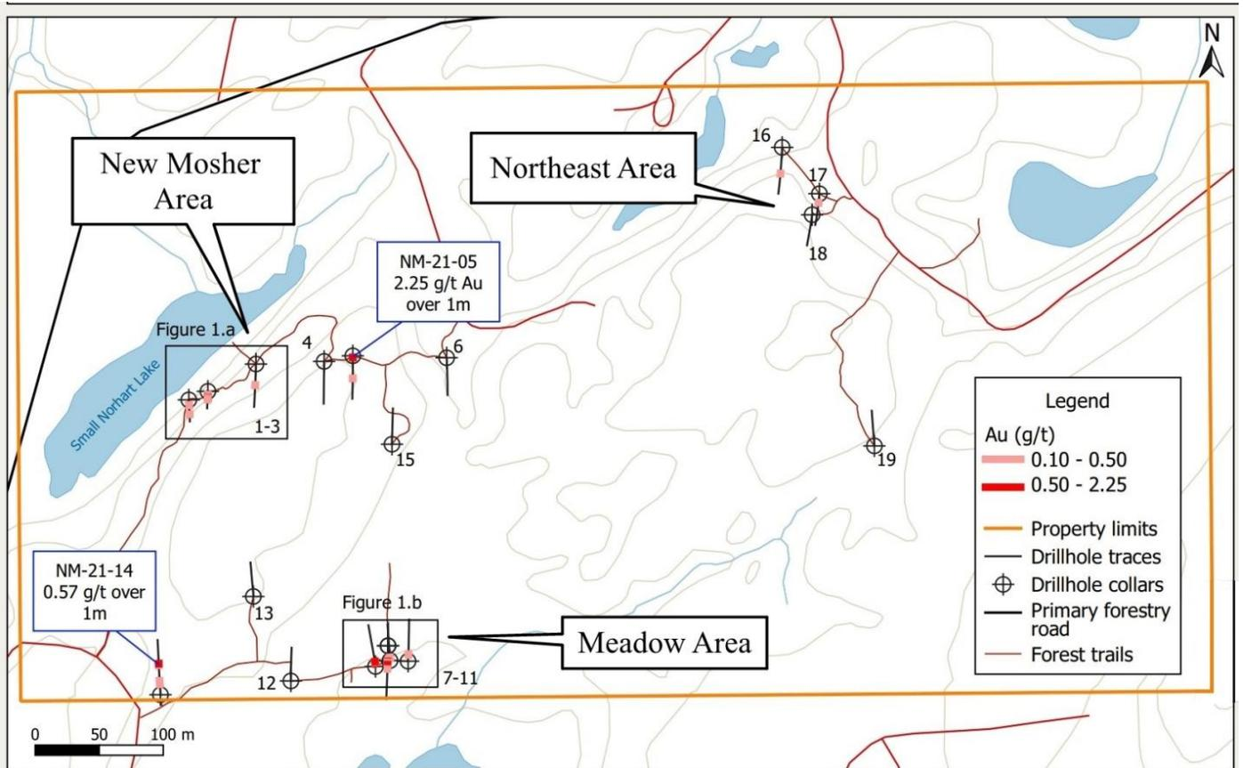
Figure 1: Diamond Drill Location Plan
