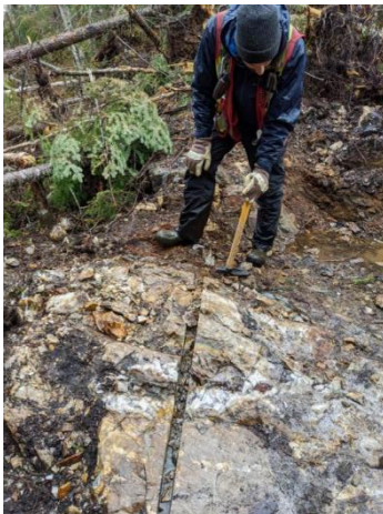
Figure 4: New Showing associated with Induced Polarization chargeability anomaly. Quartz vein in contact with quartz feldspar porphyry.
